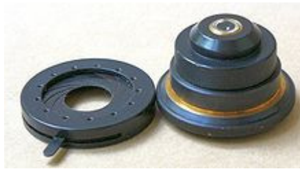
Figure 1.8: Image of a basic condenser and its respective diaphragm
