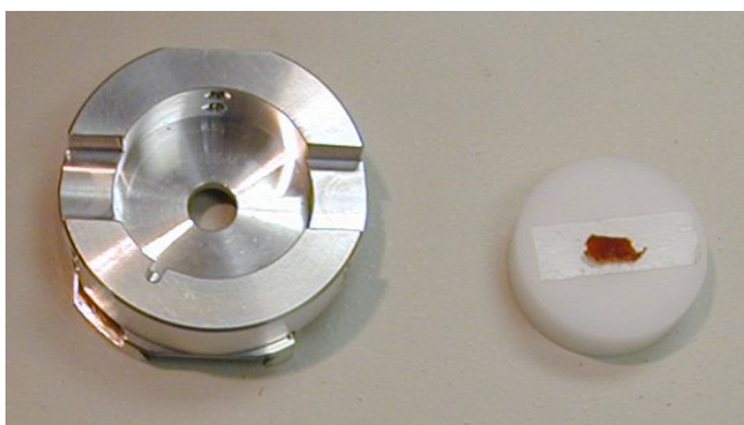
Figure 1.17 : Specimen holder in SEM
